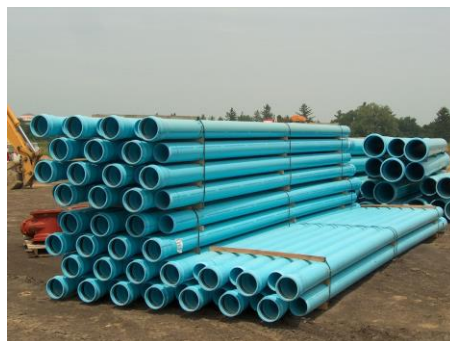
Figure 6.9: Polyvinyl chloride (PVC) pipes 48
